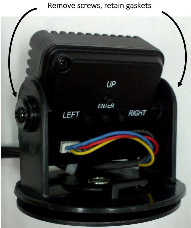
Figure 1 - ATM Camera with Plastic/Metal Bracket
